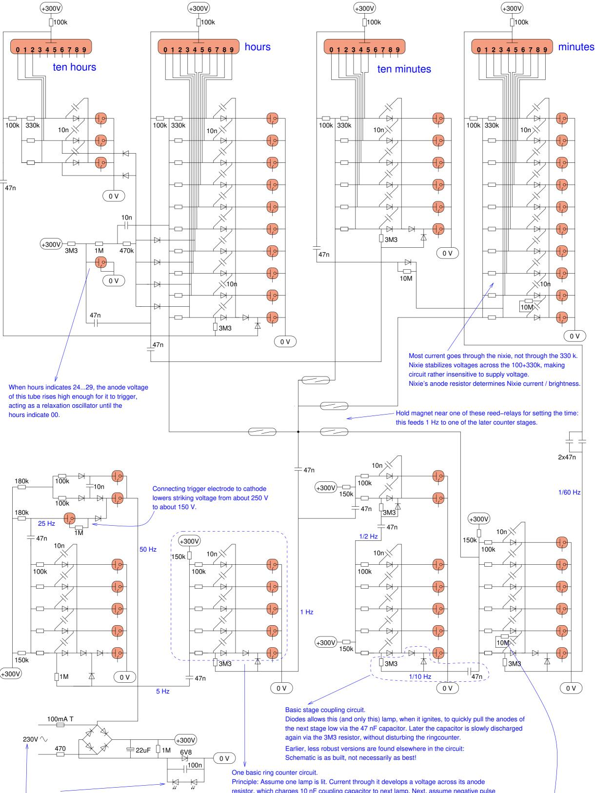
Blue leds illuminating the trigger tubes improve reliability in darkness. Neon gas discharge needs an initial ionization to get started, which can be provided by ambient light.
